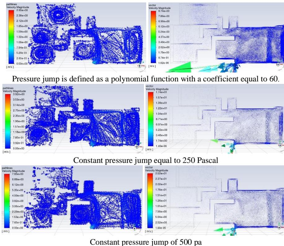
**Fig 6.** Airflow pathlines (left) and velocity vectors (right) in the indoor spaces affected by an exhaust fan with different pressure jump
