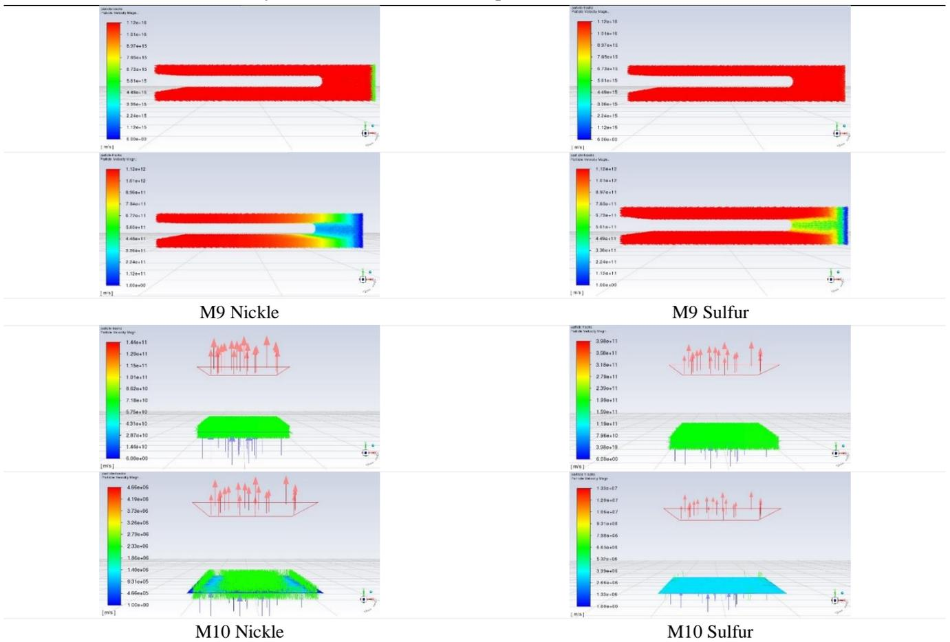
**Table 4.** The average of air velocities and temperature after passing through the coils cooled with Refrigerant and TEC
