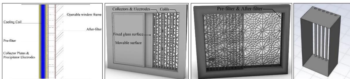
**Fig 3.** Cooling aluminum coils at the air inlet (right), and internal view and longitude section of the proposed model for the precipitator and Mashrabiya as the cooling coil (Pre-filter and After-filter are optional on both sides of the electrodes)
