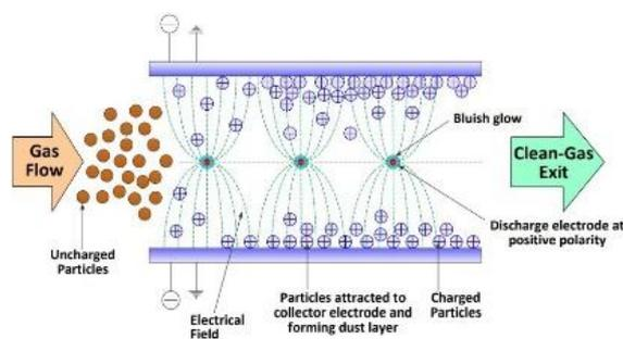
**Fig 1.** A schematic of the process of removing particles from the air in a single-stage electrostatic precipitator (Afshari et al., 2020)
