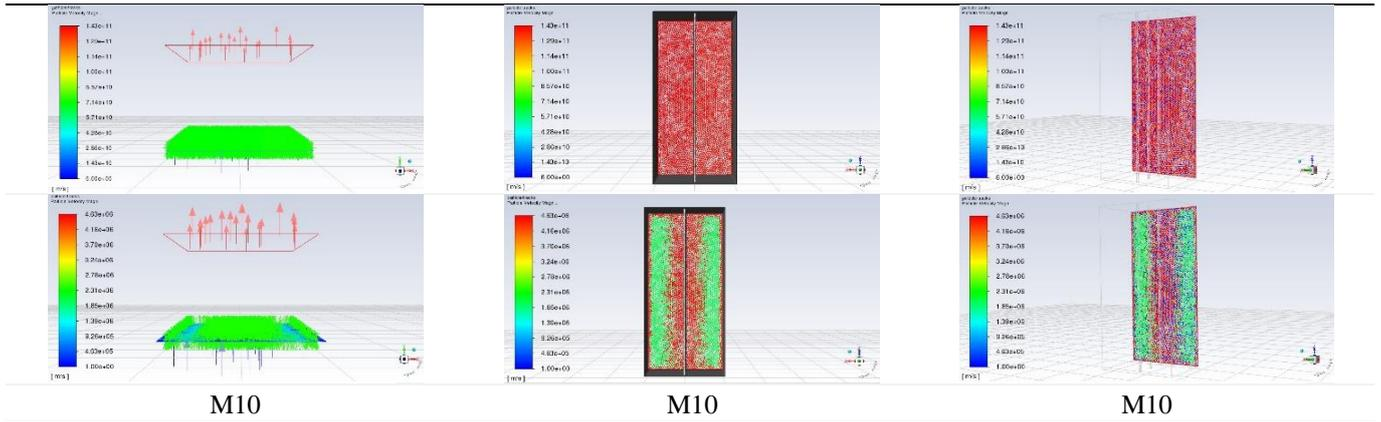
**Table 3.** The air velocity and the behavior of Nickel and Sulfur particles with a diameter of 0.1 and 10 microns at an inlet air velocity of 6 and 1 m/s, from the top view of the window in models 9 and 10
