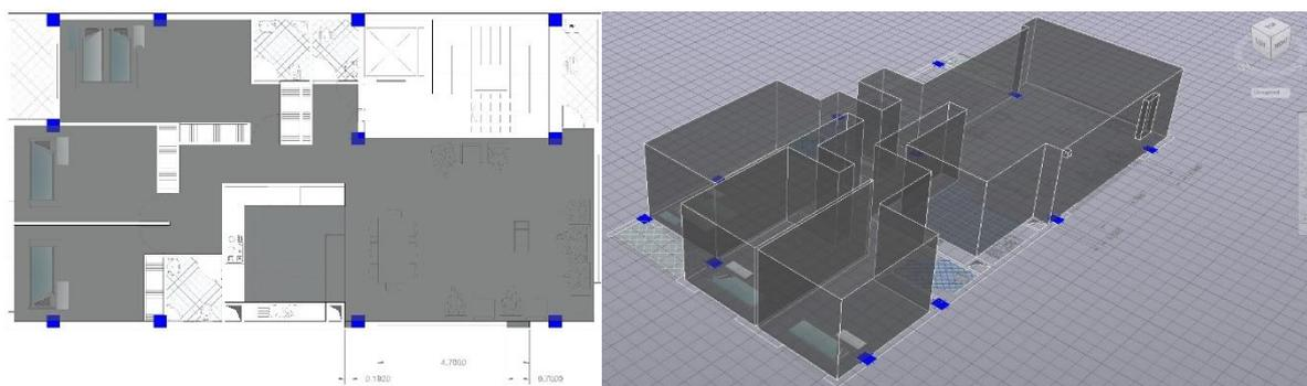
**Fig 4.** Simulated plan and volume to investigate the airflow behavior affected by the fan (The width of the window opening and the fan zone in the sitting room are 0.7<sup>m</sup> and 0.192<sup>m</sup>, respectively. The windows of other spaces were closed in the simulation).
