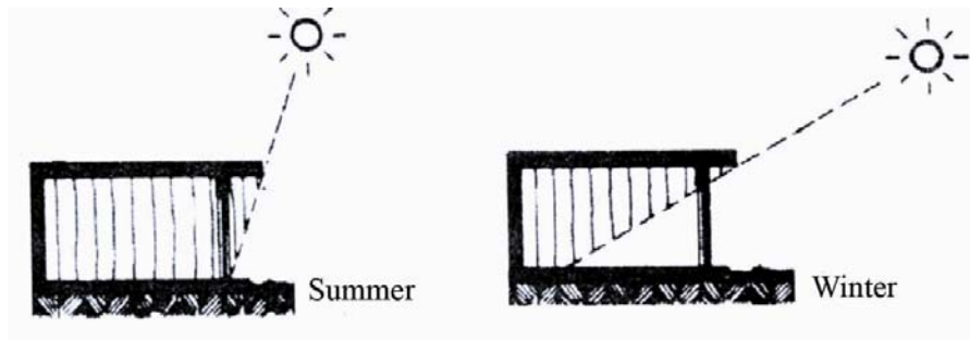
Fig. 13 Porch as a fix shade toward south front [25]
