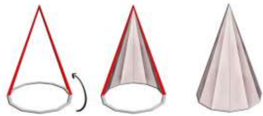
Fig 1. The Steps of the Formation of the Outer Shell of the Conical Dome through the Arch Rotation around a Polyhedral Field (Source: Authors)
