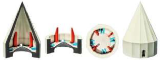
Fig 3. Graphical Representation of the Hierarchy of Poppies and Connecting Belts in the Two-layered Space of the Pyramid-shaped Rack Dome of Sultan Mirahmad's Tomb
