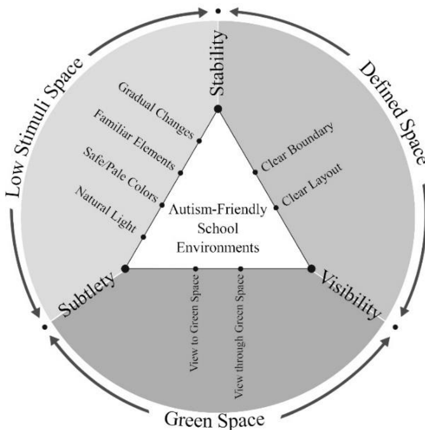
Figure 1. An autism-friendly school environment: three design concepts, three spatial needs, and eight spatial characteristics (see Table 4).
