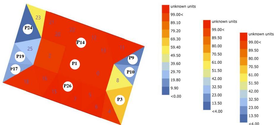
Fig 5. Simulation gride analysis and test points (including 27 general points and 9 selected points)
