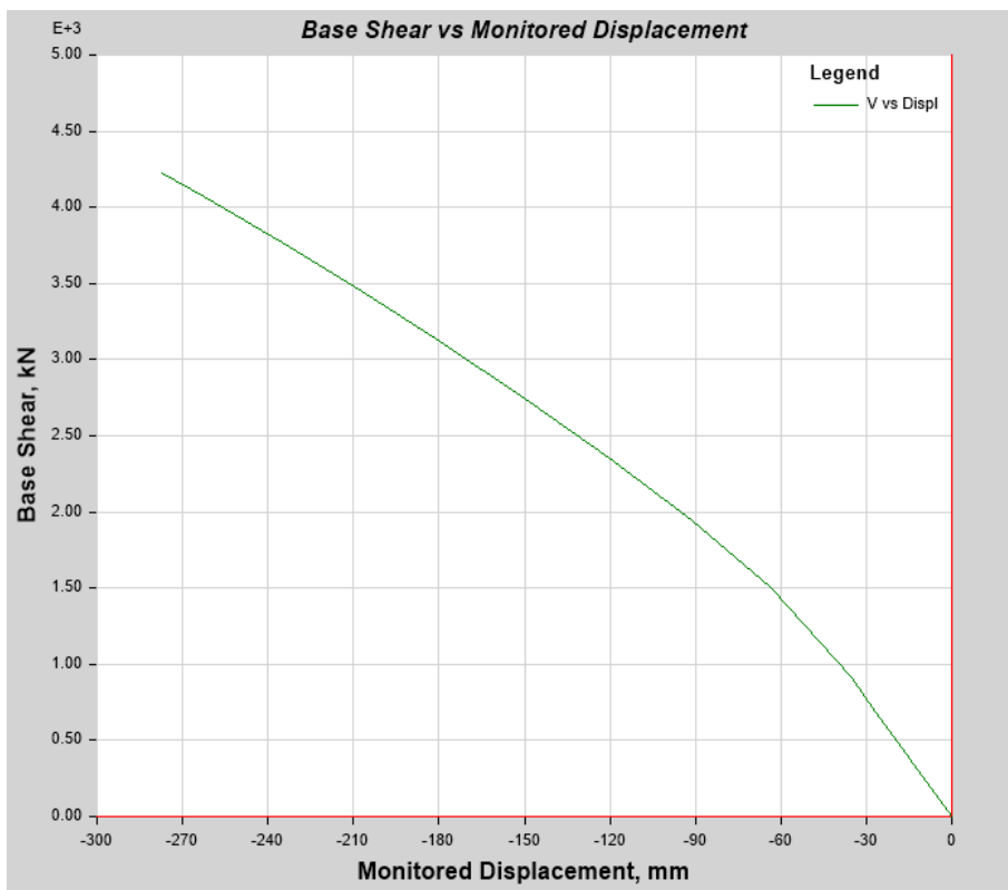
Fig 18. Base Shear vs Monitored Displacement when column section in X & Y direction is changed by 200mm
