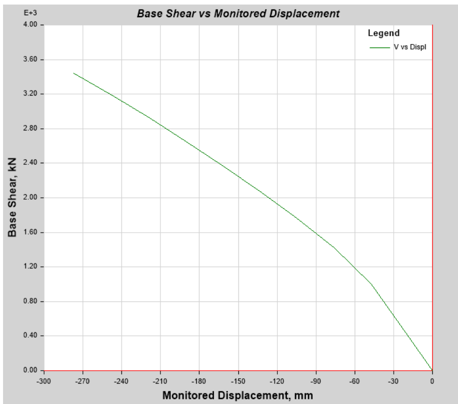
Fig 14. Base Shear vs Monitored Displacement when column section in X direction is changed by 100mm
