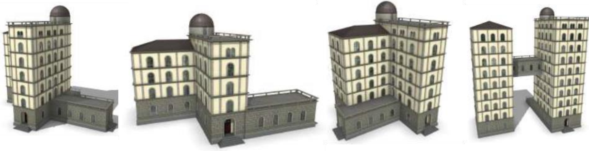
Fig.1: This figure shows the application of CGA shape, a novel shape grammar for the procedural modeling of computer graphics architecture. First, the grammar generates procedural variations of the building mass model using volumetric shapes and then proceeds to create facade detail consistent with the mass model. Context sensitive rules ensure that entities like windows or doors do not intersect with other walls, that doors give out on terraces or the street level, that terraces are bounded by railings, etc [21].
