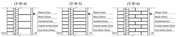
Figure 2: Details of insulated exterior walls' structures.
