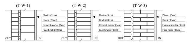
Figure 1: Details of none-insulated exterior walls' structures.
