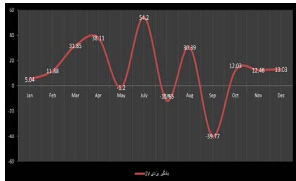
Diagram 2: Air flow velocity in the openings Yazdi wind towers [Authors]
