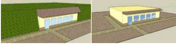
Fig. 9. The analyzed schemes of earth-sheltered and above-ground buildings [5].
