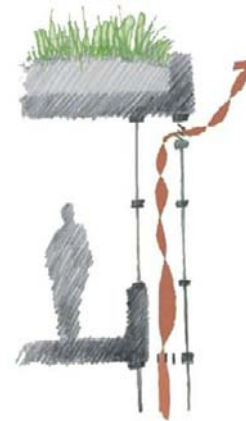
Fig. 4 The idea of DSFg system with vertical ventilation to decrease the greenhouse effect in summer [9]
