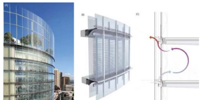
Fig. 10 (A and B) The double-skin façade of 1 Bligh Street has a system of internal blinds that automatically deploy or adjust to optimize the combination of daylighting and energy transmission while protecting the occupants from glare. (C) Detail of air movement through the façade. [38]
