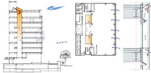
Fig. 6 Natural ventilation concept for the Sekisui Building office tower in Tokyo Japan; combined the wind and ventilation across DSFg [26]
