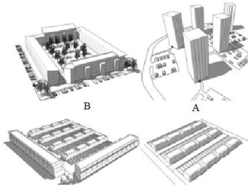
Fig 5. Residential complex layout (A) Point, (B) Central, (C) Linear, (D) Mixed [25]
