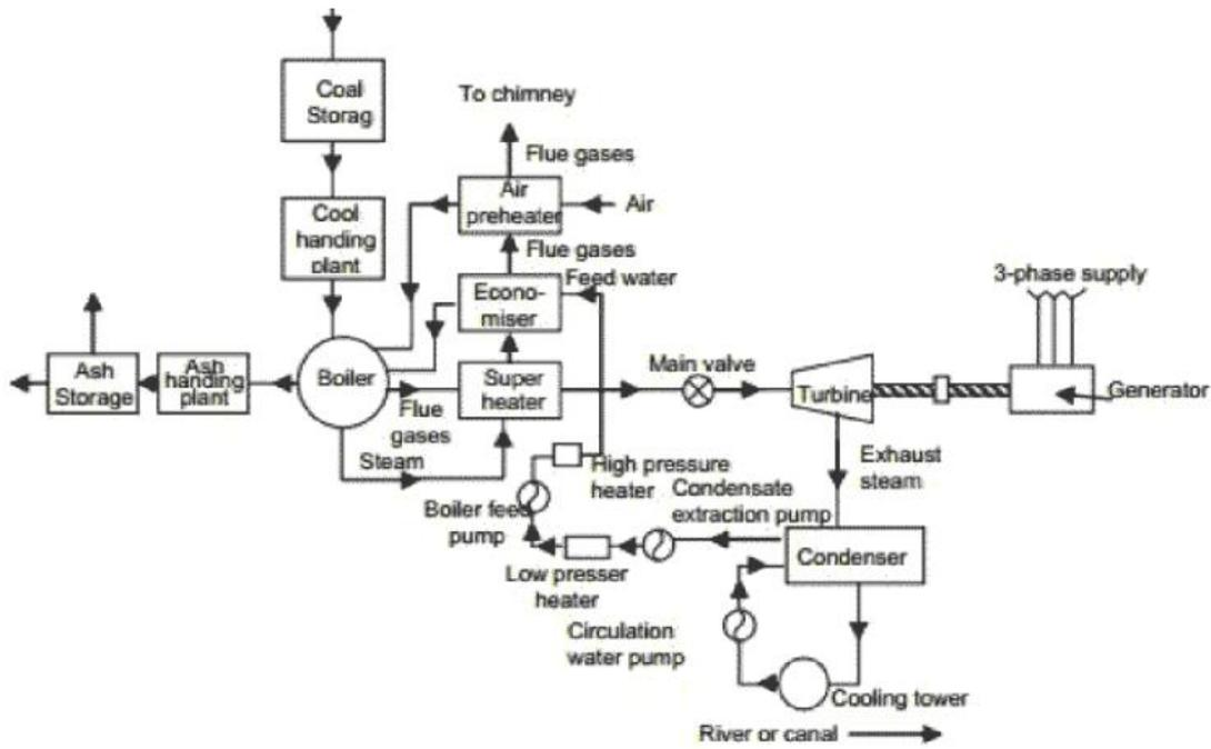
Fig. 1 Block diagram of thermal power plant [12]
