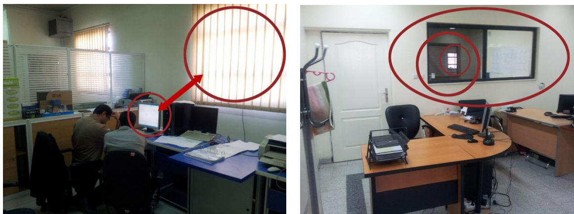
Fig. 6 The picture on the right- arrangement of office furniture in engineering room is not in accordance with the windows. The curtain is not properly selected for uniformity and fragmentation of incoming light from the windows The picture on the left- the administrative office lacks external windows. For improving the enclosed interior conditions false windows have been embedded. Using white electrical lighting has intensified the interior adverse conditions. Source: authors
