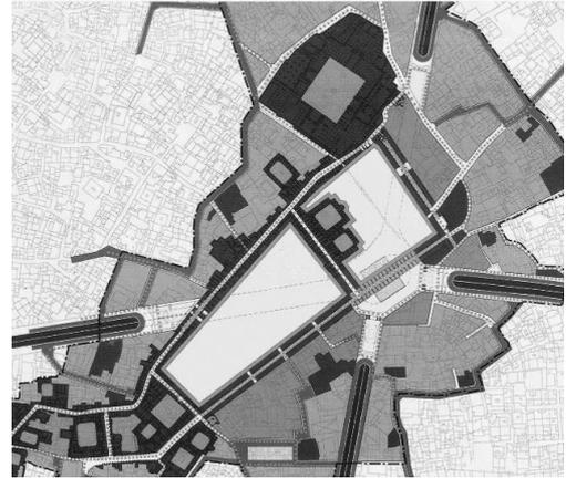
**Fig. 3b** The situation of the square after its revitalization and construction of the underpass in 2008. Having constructed the underpass in the area of the square and transferring Abdolrazagh Street to underground level, structural-historic integrity in the area of the Isfahan historical bazaar was provided. The square form was returned to its original one and was very effective in providing the visual integration of the area of the square and its connection to Isfahan bazaar [24]
