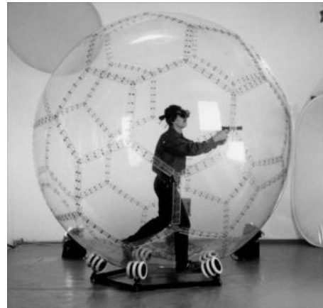
Fig. 4 Using a Virtusphere can create high levels of immersion in virtual environment. Source: [17]
