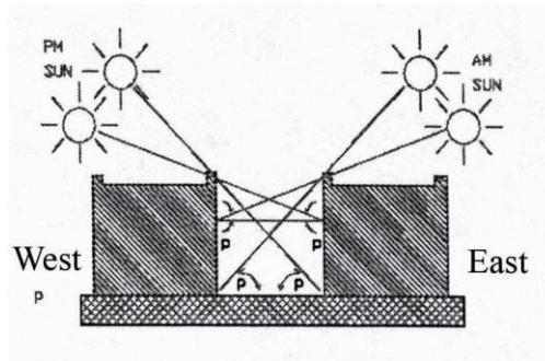
Figure 8- The impact of H : W dimensions on shade and sun in open spaces, [19]
