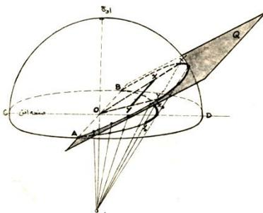
Figure 4- Stereograph of a direct horizontal line shade mask,[16]
