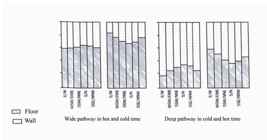
Figure 6 –Solar energy received by floors and walls
