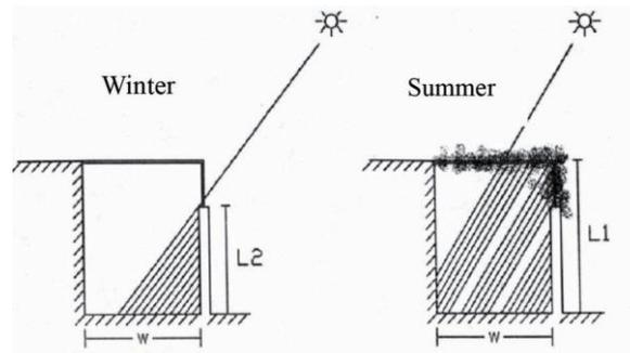
Figure 10- Using trailing plants as a temporary horizontal shade ( $L1 < L2$ )
