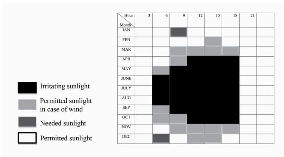
Figure 3- The times that shade and sun are required in open spaces of Yazd (Yazd meteorological station data (1952-2000))
