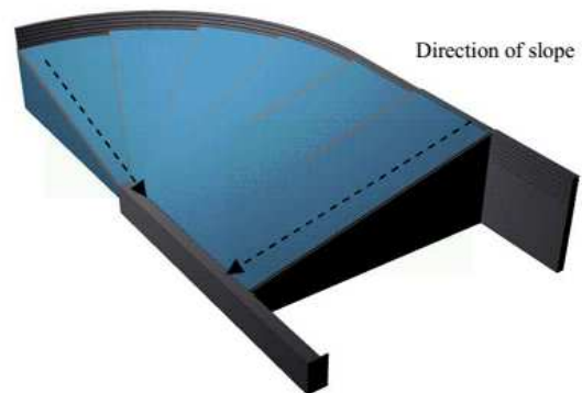
Fig. 7. Slope of 25% in each panel toward edges
