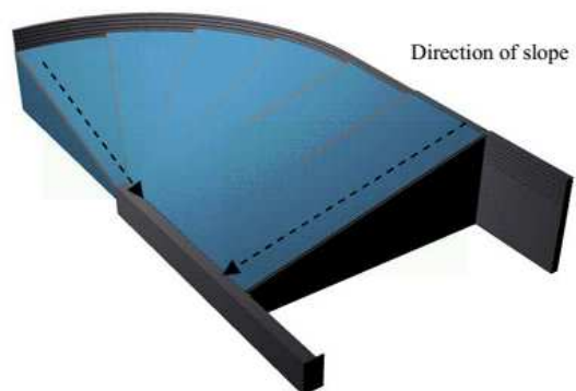
Fig. 7. Slope of 25% in each panel toward edges
