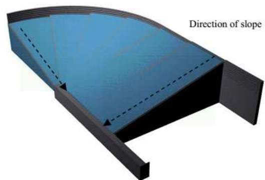
Fig. 7. Slope of 25% in each panel toward edges
