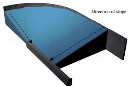
Fig. 7. Slope of 25% in each panel toward edges
